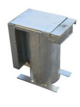
Built-in metal support for the hollow bollard. It allows the removal of the bollard if necessary. It works with a universal key (included). Measurements: 21.5 cm long x 14.5 cm wide x 26 cm high.
